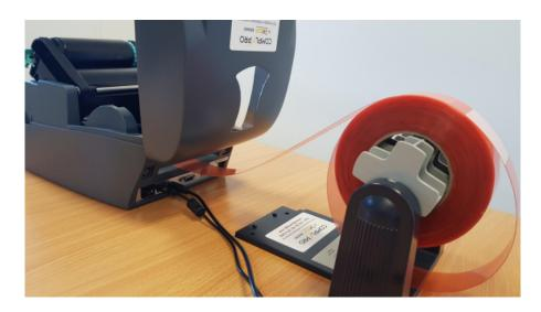
b. Feed Hose Wrap Material under Ribbon Carriage and out the front of the cutter/ printer.
