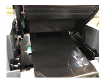
d. Place Cardboard Take-Up Core on front side of ribbon carriage and attach ribbon.
